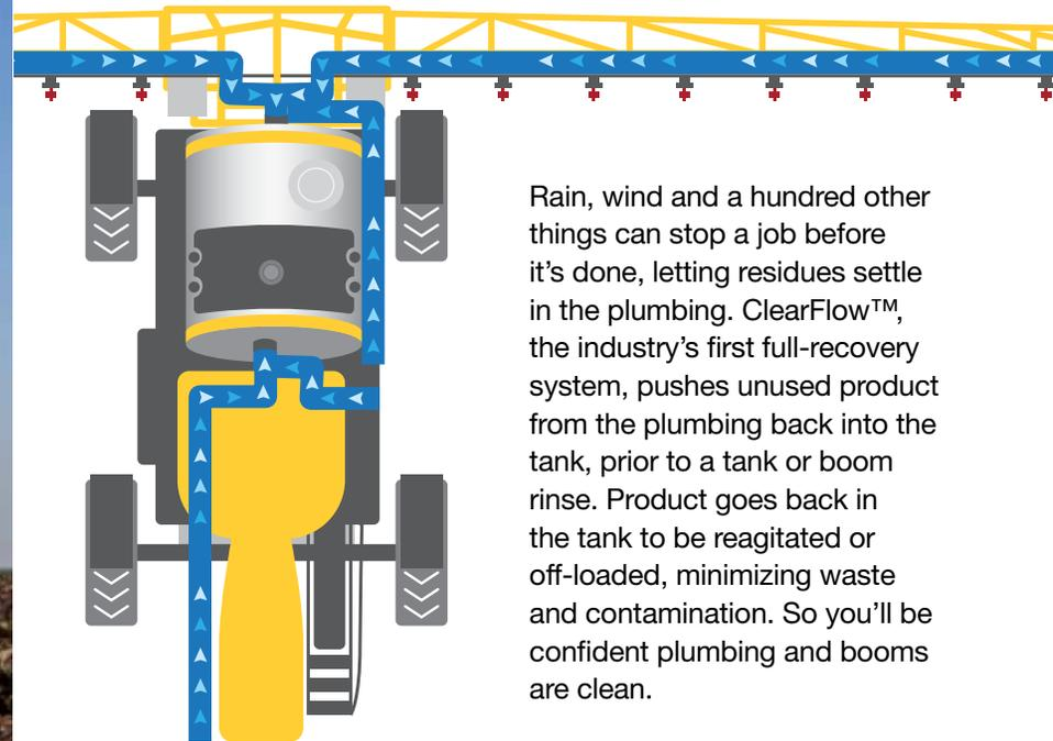
Rain, wind and a hundred other things can stop a job before it’s done, letting residues settle in the plumbing. ClearFlow™, the industry’s first full-recovery system, pushes unused product from the plumbing back into the tank, prior to a tank or boom rinse. Product goes back in the tank to be reagitated or off-loaded, minimizing waste and contamination. So you’ll be confident plumbing and booms are clean.
