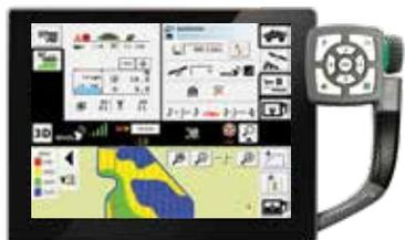
**RATE AND SECTION CONTROL** AgControl rate and section control lets you control up to 36 sections with tip-to-target accuracy, and seamless integration between software, pump, plumbing system and all chassis functions. Or control up to 16 sections with the optional Raven® Viper® 4 controller.
